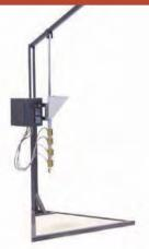
**INJECTION MACHINE:** It heats plastic flakes and is ideal for recreation of small projects with injection moulding.
