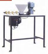
**EXTRUSION MACHINE:** This machine creates a continuous line of plastic and can be used to create 3D-printing filament.
